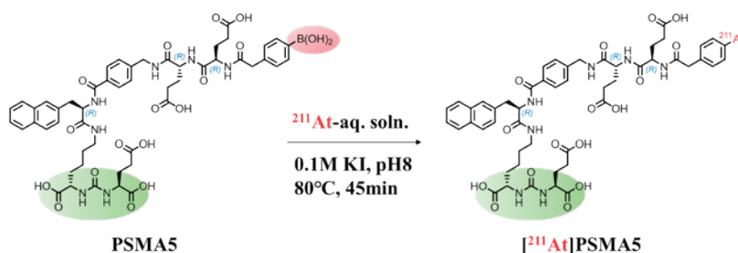
Fig. 1 Chemical structure and radiolabeling scheme of [ 211 At]PSMA5
